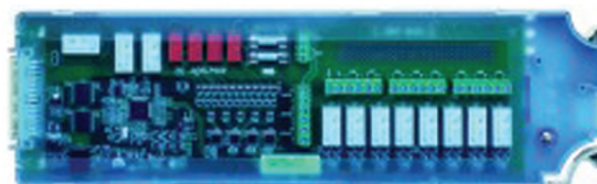
DAQ-919 8 CHANNEL DC 1000 V / AC 750 Vrms voltage
