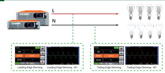
AFV-P series provides optional LED TRIAC Dimmer function, which can simulate output of TRIAC dimmer. The user can select whether to perform LEADING EDGE DIMMING or TRAILING EDGE DIMMING via HMI. Compared with traditional TRIAC dimming, the output waveform can be controlled more accurately and effectively.
