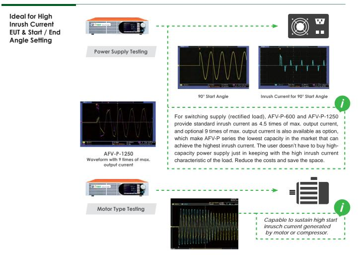
The AFV-P series can provide up to 4.5 times of peak current from its maximum rated current, which is ideal for inrush current test, such as electric motor test. Additionally, the AFV-P series allows user to set the start angle/end angle for the product output, which is suitable for testing switching power supplies.
